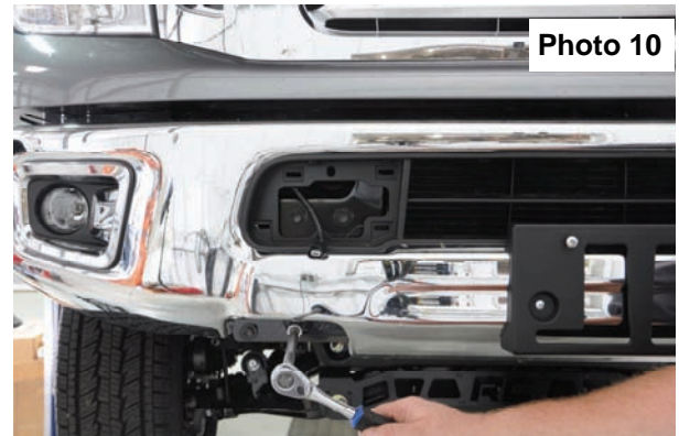
Remove the front bumper mounting bolts.
