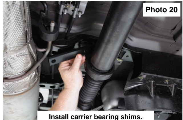
Install carrier bearing shims.
