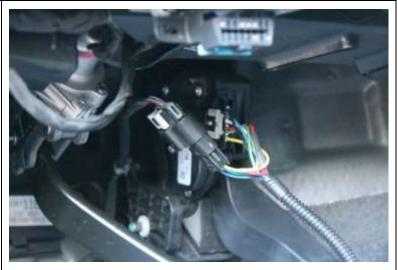
Before mounting the module, open the module by inserting a screwdriver to depress the tabs and slide the PCB from the enclosure.
