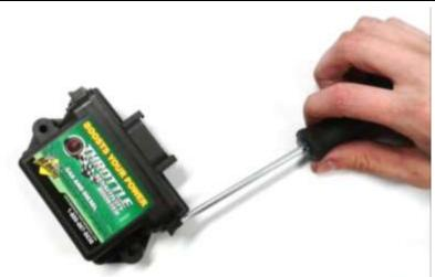
Connect circuit board to the wiring harness and keep away from metal objects that might cause a short circuit. Ensure the sensitivity "SETTING" switch is set to the default position of "STOCK".
