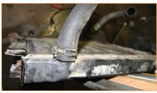
**5.** Using your hose clamp pliers or channel lock pliers, remove the lower radiator hose from the vehicle. (Note: For automatic transmission vehicles, you must remove the two transmission cooler lines at this time. Place a drain pan below as fluid may leak once the lines are removed.)
