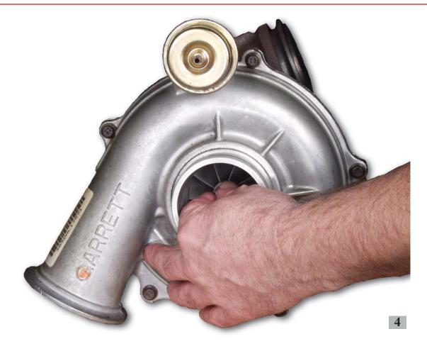
Spin the compressor wheel to make sure that it spins freely. The wheel should not contact the housing.
