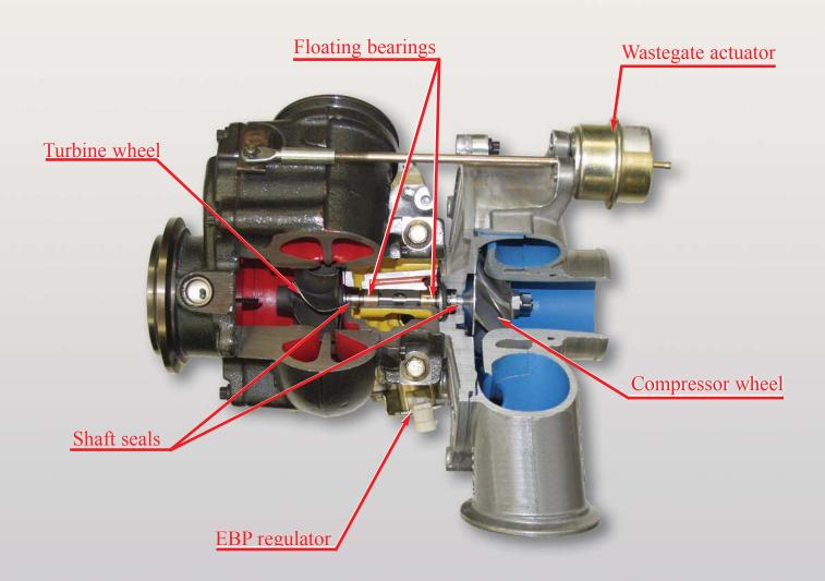
Turbochargers are precision pieces of machinery which operate at high speed, using heat of expanding exhaust gasses to "boost" intake manifold pressure. Turbochargers increase performance and decrease exhaust smoke through improving an engine's volumetric efficiency.
