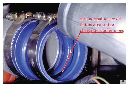
Normal Oil Carryover: The photo to the left shows normal oil carryover in the charge air cooler pipes. This condition can be aggravated by excessive air inlet restriction. The turbocharger should not be replaced for this condition.
