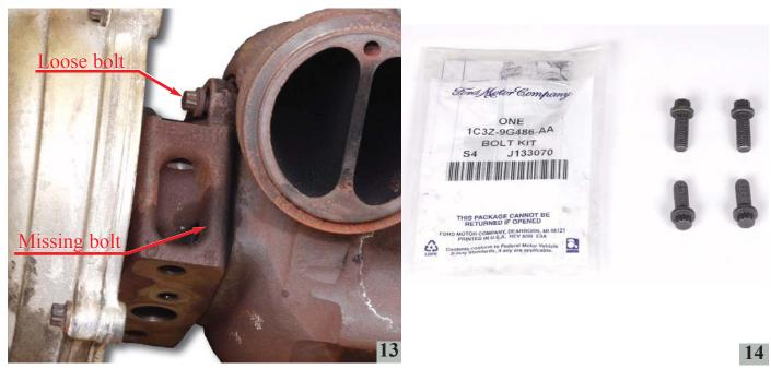
When loose or missing bolts are found, replace the bolts with part number 1C3Z-9G486-AA per TSB 03-14-09.
