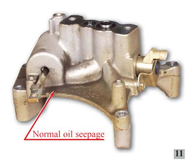
**Normal Oil Seepage:** It is normal to see some oil seepage past the seal on the EBP actuator rod. The photo to the left shows this normal seepage.
