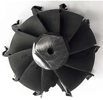
**Structural Failure:** Above right is a turbine wheel that has failed due to overspeed as a result of performance modifications.
