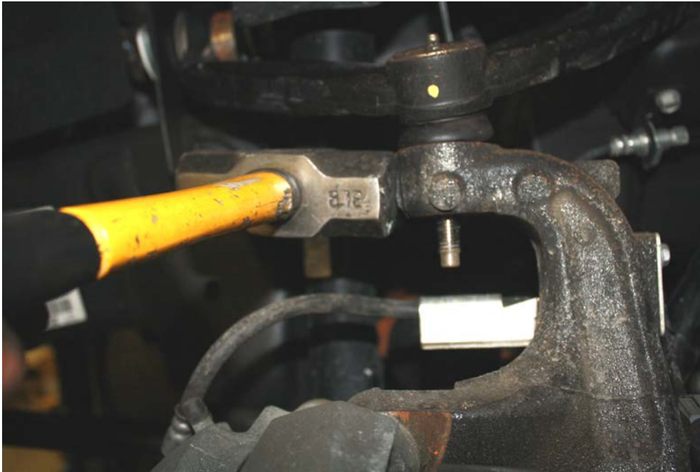
Figure 1: breaking ball joint loose from spindle
