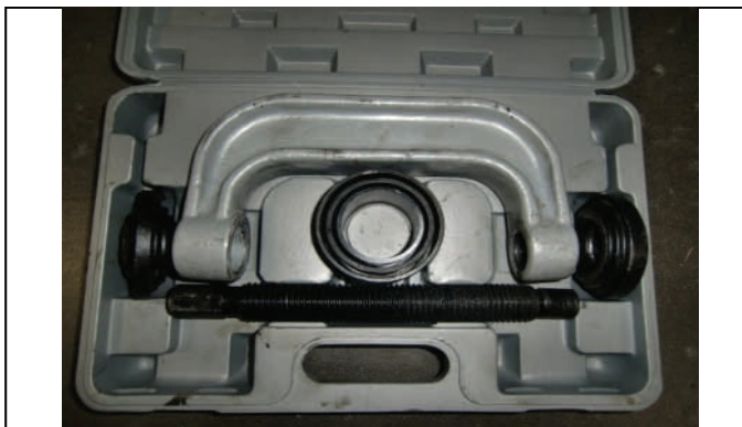
Use proper heavy duty ball joint removal tool set.
