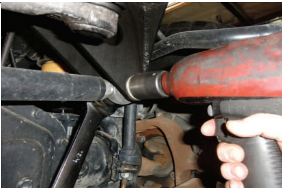
Tighten other end at the frame mount to OE spec.
