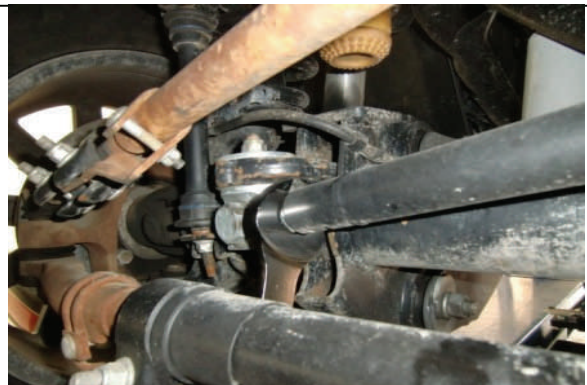
Tighten jam nut at axle mount and at frame bracket.
