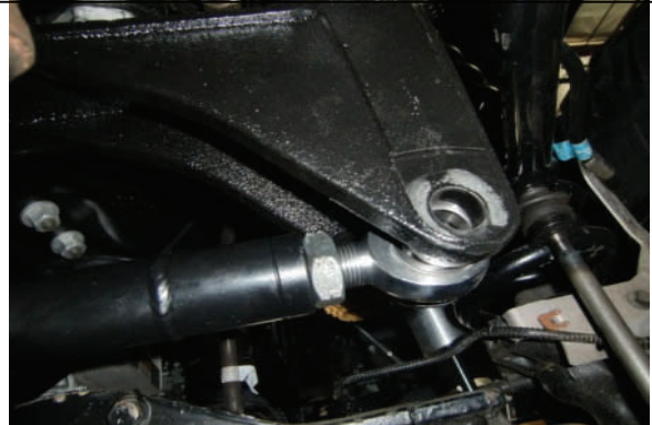
Position other end at frame w/ provided misalign spacers
