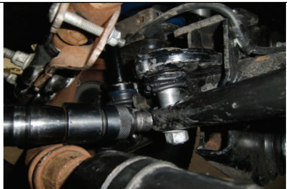
Use ball joint fork/air hammer to separate bar from ball joint
