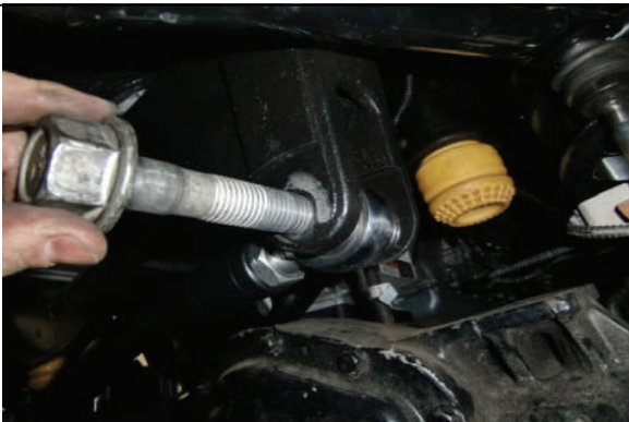
Attach with original hardware, and check track alignment
