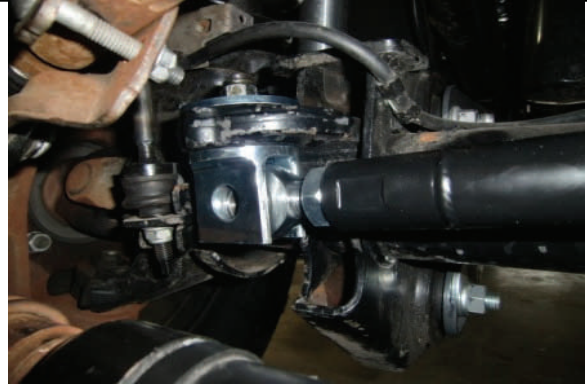
Insert track bar into clevis, check clearance again.
