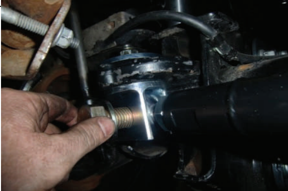
Attach with provided hardware, do not tighten until adjusted
