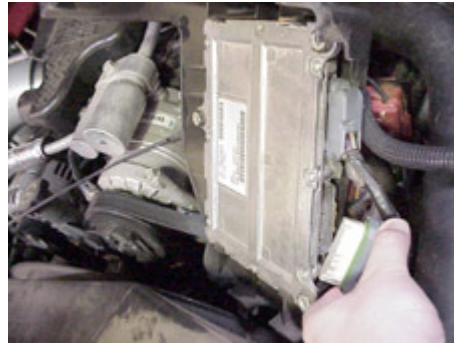
Figure 17: Removing electrical connector
