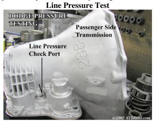
Tape the gauge to the outside of the windshield; this is a precautionary measure to ensure you do not have an accident in the event there is a hydraulic leak. First bring the transmission and engine to full operating temperature, then note the line pressure at idle in neutral. Be sure the
