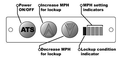
Figure 1: Co-Pilot Face Plate Configuration
