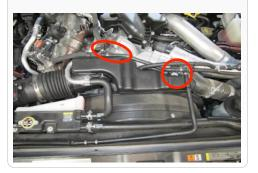
7. Remove the air box by carefully pulling it up out of the OE grommets. Be sure the grommets remain in position for the S&B installation
