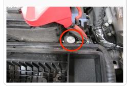
$9. \ {\rm Install \ the \ air \ inlet \ gasket \ onto \ the \ Air \ Box}$ (A). Push the two prongs into the holes located on the bottom of the Air box.
