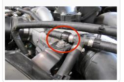
23. Install the Insulation Tube (Q) around the factory coolant hose by removing the protective film on the adhesive and sticking the two sides together.
