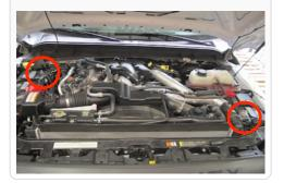
4. Loosen the clamp at the turbo inlet and remove the bolt securing the resonator tube to the shroud.
