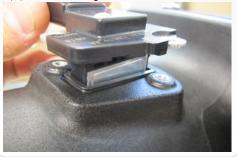
16. Install the Intake tube assembly into
