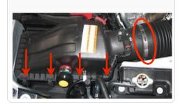
3. Loosen the hose clamp at the intake tube
