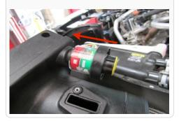
15. Install the Hump Adapter (K) over the Intake Tube (C) using the remaining two #72 Hose Clamps (L) until it is nearly flush with the end of the tube.
