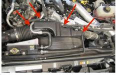
$\mathbf{8}$ . Remove the air inlet gasket from OE air box
