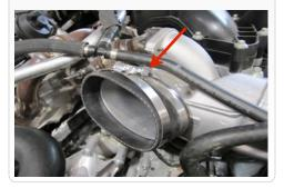
**17.** Install the Air Filter (D) onto the Adapter Tube (B) and tighten the #80 Hose Clamp (E).
