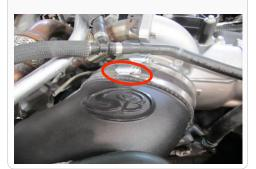
19. Slide the Hump Adapter (K) over onto the Adapter Tube (B) and tighten both #72 Hose Clamps (L).
