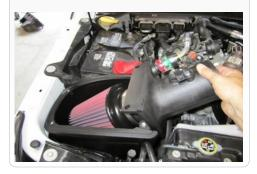
$\label{eq:21.Reconnect the wiring harness to the MAF sensor.}$
