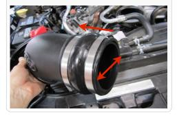
**18.** Carefully install the Filter/ Adapter assembly in the Air Box (A).
