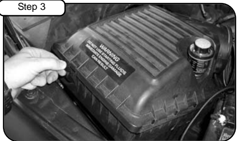
Un-clip upper half of air box and remove.
