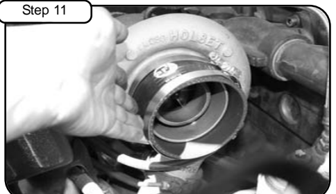
Install high temp coupler to turbo using clamps provided. Do not tighten.
