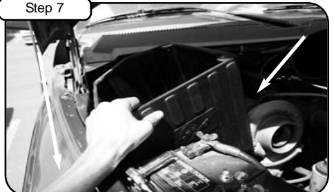
Install housing into vehicle and position.
