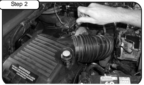
Use 5/16" nut driver to loosen clamps on OE tube at turbo/air box and remove.
