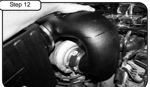
Attach 6" hump coupler with clamps provided to tube and install tube to turbo and filter adaptor. Adjust and tighten all clamps with 5/16" nut driver.
