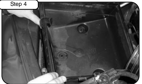
Carefully lift and pull bottom half of air box to remove from vehicle.
