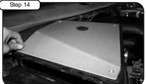
Install cover and tighten using button head screws provided. Tighten with 5/32" allen key.
