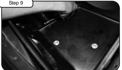
Secure housing using fender washers and nuts provided. Tighten using 7/16" socket or wrench.
