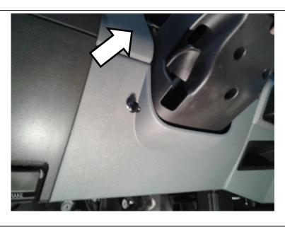
12. Drill a 7/8" hole in the dashboard with a stepper bit or hole-saw. Using a small file, create a notch for the locator tab of the switch. Clean up the edges of the hole as necessary with the file.
