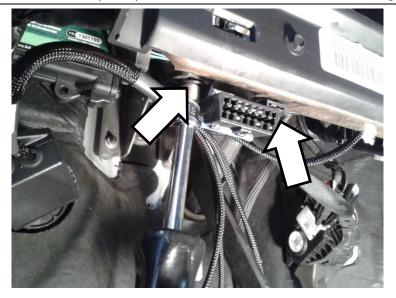
Install the OBD connector from the BD VVB kit in place of the original and reinstall the screws.
