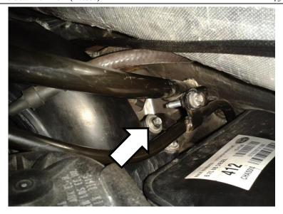
23. Remove the 15 fasteners from the intake manifold. These are 8mm screws. Remove the manifold from the engine.
