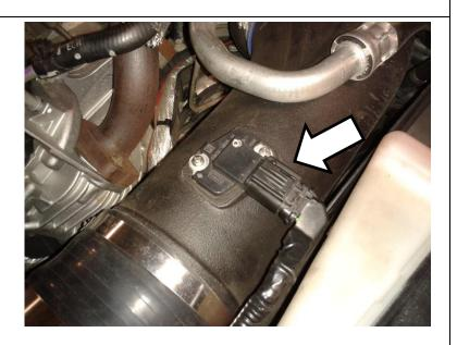
28. Connect the BD VVB harness inline to the MAF sensor and to the stock wiring harness.
