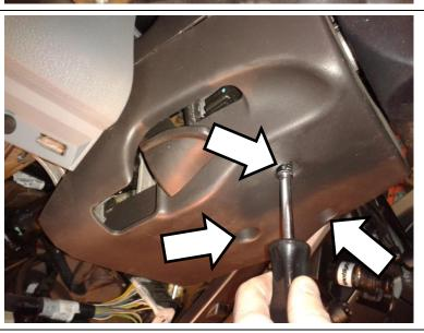
6. Pull the steering column covers apart and remove top cover.
