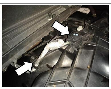
21. Disconnect the coolant tube hold down clip from the intake manifold.
