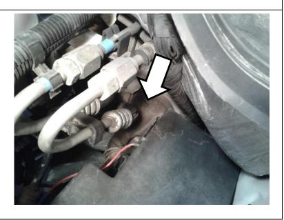
16. Connect the engine bay wiring disconnect to the in-cab wiring harness.
