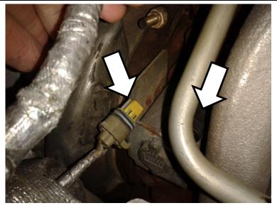
25. Connect the BD VVB wiring harness to the turbo solenoid and to the OE wiring.
