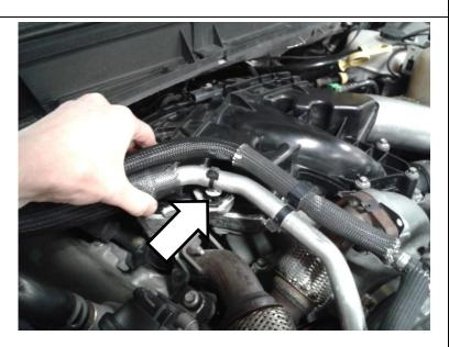
22. Undo the transmission and engine oil dipstick tube bracket from the intake manifold by removing the 8mm fastener.
