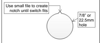
Install supplied switch decal onto the dash aligning the notch on the decal with the notch you created. Then install the switch into the hole.
