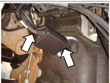
5. Remove the three 5.5mm screws from the bottom of the steering column cover.
