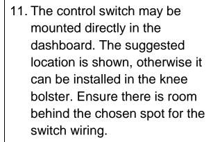
**Note:** If the installer prefers to mount the switch below the dash, a metal bracket is included.
