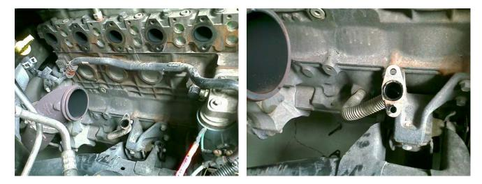
Next. Locate the front freeze plug (same height as the back oil drain port). Take a punch or screwdriver and lightly tap on one edge of the freeze plug to get it to rotate or twist inside the hole. Then take a pair of needle nose pliers and remove the freeze plug (BE VERY CAREFUL NOT TO PUSH THE PLUG INTO THE OIL PAN, OR YOU WILL HAVE TO DROP THE OIL PAN TO RETRIEVE IT).
