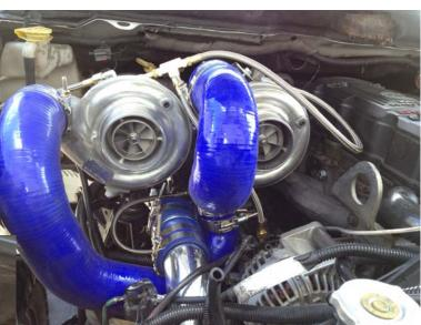
11. Attach the rubber oil drain/return line to the fitting you tapped into the engine earlier. Then attach the oil drain lines of the two upper turbos to the 'T' where the oil drain lines come together. Make sure the 'T' and is below the bottom of the turbos, and the drain lines slope down.
