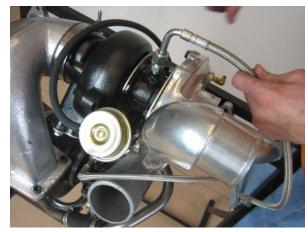
Next, remove one of the oil plugs from the top of the oil filter mount, and screw in the provided fitting (should be at the end of the steel braided oil line from the large turbo), then couple the oil line to that fitting.
