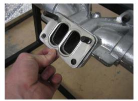
You will need to remove the mounting studs from the turbo, and drill out the threads from the two threaded holes in the turbo. Use one of the following size drill bit size 'X', 'Y' or 13/32, to drill the threads out.
