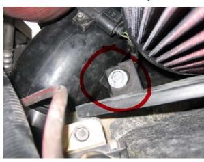
17. Install **both** stock sensors into the rubber tube, install the air filter.
