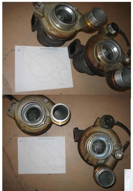
These two pictures show stock turbos. The turbo on the right is the stock clocking. The turbo on the left has been clocked according to the template.
