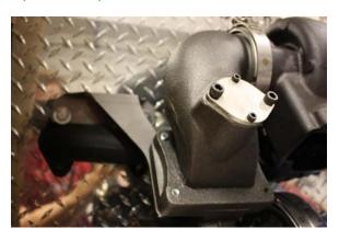
Tighten the bolts most of the way, but do not completely tighten theses two bolts...yet.
