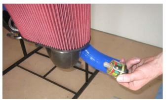
18. Attach the metal fitting which is in the end of the silicone tube first to the large turbo air outlet.
