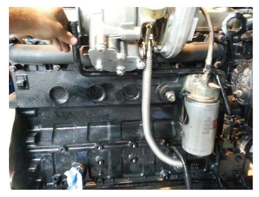
Top Turbo Oil Drain will go in as shown here
