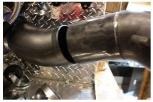
16. Install large rubber hose with steel ends, as shown. The ear shown below should align with the ear on the side of the battery box. If it does not, the two rubber boots should be clocked/twisted differently or the cast iron elbow may need to be clocked differently.
