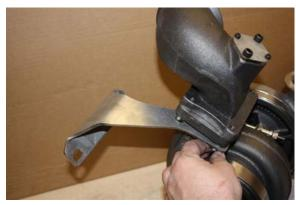
Leave the two bolts going through the bracket just barely loose, so they can be adjusted, once the top is on. All of the bolts going through the support bracket should be a little loose to allow the lower turbo to be adjusted to align the hot pipe with the top turbo. If necessary the bracket can be slightly flexed during the installation if the bolts are a little loose, then tightened when everything is aligned.
