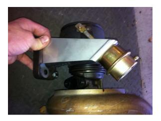
WASTEGATE (ABOVE): The new supplied wastegate actuator and bracket will be mounted as shown above. When the turbo is mounted on the manifold the mounting bolts will be used to hold this bracket in place.
