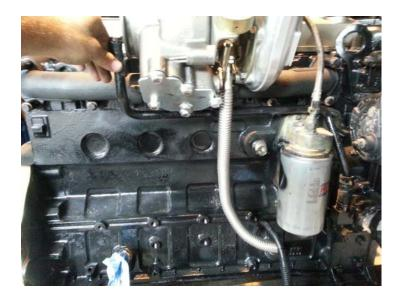
**8.** Find the 4.4 inch v-band clamp that connects the small turbo to the hot pipe (elbow). Remove the nut off the v-band clamp or simply unhook the bolt so the clamp is open, and set the open clamp on the rear of the small turbo's flange where it will mount. On the stocker kits you should already have an adapter and clamp that is pre-attached to the hot pipe.
