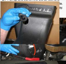
7. Prior to installing the Air Box (A), you may need to rotate the factory intercooler clamp that is located just below the OE air box to add clearance for the new one
