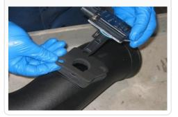
17. Place the factory grommet from Step 6 into the intake tube and insert the grommet completely flush into hole. Insert the restriction gauge into the grommet on the intake tube. Make sure the gauge is inserted completely into the grommet of the intake tube.
