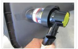
3. Depending on your vehicle year, disconnect either the MAF sensor or the Temp. sensor electrical connection on the OE intake tube.
