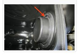
22. Slide the Coupler Adapter (N) over the short intake tube and center over the gap.
