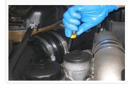
24. Carefully place the Air Filter (D) into the Air Box (A). Attach filter to intake tube and tightened down firmly.
