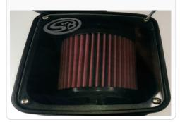
28. For those concerned about minimal engine heat; leave the Clear lid installed (G) on top of the Air Box (A). For those seeking additional air flow, Install and bolt on the Top Inlet Lid (See below for more info)
