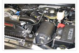
If Equipped: Disconnect the electrical connection at the OE restriction gauge located at the back of the air box.
