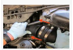
23. Secure both #72 Hose clamps after both tubes and coupler are aligned together straight.
