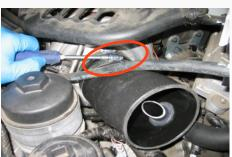
tube then secure using a #64 hose clamp (F).
