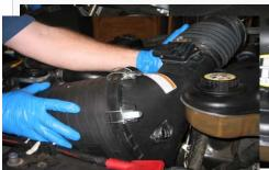
4 (A). If you have the OE "Two Piece" intake tube, loosen the hose clamp at the bellows.
