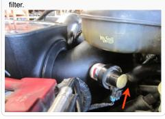
**26.** Reconnect the electrical connector to either the MAF sensor or Temp. Sensor located on top.
