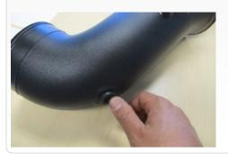
18. Slip the Hump Adapter (N) along with two #72 hose clamps (V) over the Intake Tube (C) until nearly flush with the end.
