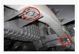
9. Insert the supplied Grommet (D) into the Air Box (M).
