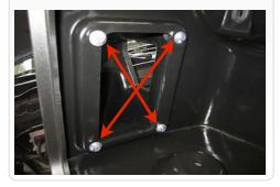
11. For those concerned about minimal engine heat; insert the Air Inlet Plug (T) into the end of the Air Inlet tube (S). Attach using the supplied 1/4"-20x3/4" screws (V), 1/4" Lock washers (U) and 1/4" Flat washers (W). For those seeking additional air flow, set the Air Inlet Plug aside and save all the supplied hardware. (See page 3 for more info and test results)
