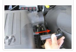
5. Remove air box by carefully pulling the air box up out of the four pins in the air box tray. Then remove the two bolts mounting the tray to the frame using 13mm socket.
