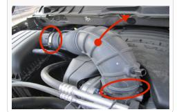
4. Remove the crank case vent tube from the air box
