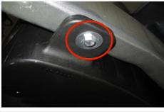
16. Reinstall the wheel liner using 5 of the OE screws and 3 supplied Panel Pins (Y). Reinstall wiring harness connector into wheel liner that was removed in Step #7.
