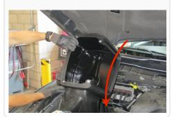
14. Using the OE bolt, secure the air box assembly to the frame. Leave loose for now. Secure the A/C line assembly if it was loosened in Step #12.
