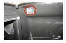
15. From inside the wheel well, attach the air box to frame using the supplied M8 x 40mm Hex bolt (K) and Fender Washer (L). Then secure both bolts mounting the air box to the frame.
