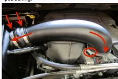
24. Reconnect the Temp. Sensor wiring harness.
