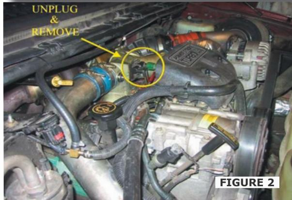
**STEP 2** – Unplug the red vacuum line from the wastegate actuator and trace it back to the Y-pipe (fig2). Here you will find a bracket with a single bolt holding it to the Y-pipe. Remove this bolt, unplug the green harness connector, and remove the assembly (with green and red lines still attached) from the engine. Be careful not to bend or break either line while removing this assembly.
