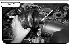
With 5/16" nut driver loosen clamps on OE tube at turbo/air box and remove. Loosen clamp at turbo and disconnect crank case line with pliers. Remove tube.
