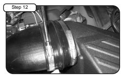
Tighten clamps at upper-cover with 5/16" nut driver.
