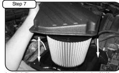
Install air filter to cover housing, tighten using 5/16" nut driver. Place cover to bottom of housing and set to posi-
