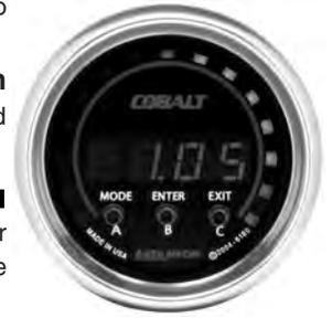
**Bar Graph Forward High Setting:** The bar graph forward high mode allows you to adjust the G force scale for forward acceleration as shown on the D-PIC when operating on the forward axis in Real Time mode. For example, if you set the **BFH** to 1g, when the bar is fully lit on the right hand (acceleration) side, the vehicle is achieving 1g of acceleration force or more.
