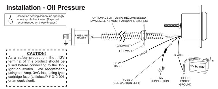
**NOTE:** Some late model vehicles use electronic sensors in their pressure and temperature senders for engine control functions. Before removing the original sender, we recommend that you contact your automotive dealer to be sure no critical functions will be disrupted.
