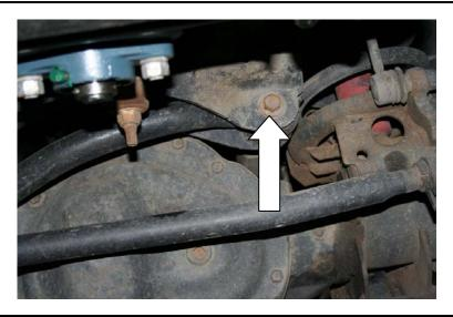
Using the 18mm socket remove the passenger side track bar bolt. Again you will re-use for reinstallation.
