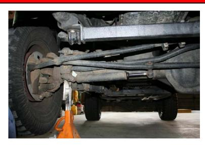
Using an 18mm socket remove the driver's side track bar bolt. You will reuse this bolt for reinstallation.
