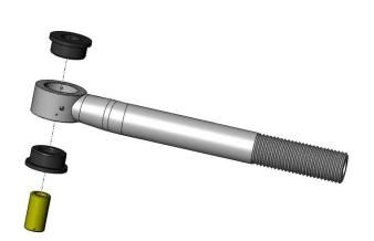
Locate the driver's side track bar section (#1302030-1). Thread the straight grease nipple (#1302057) into thread port on the side of the unit.
