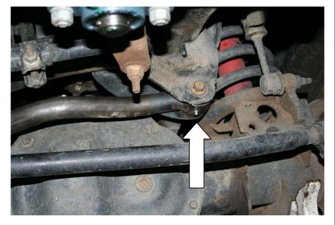
You can now perform an alignment on the front end of the vehicle. Adjust the front axle left and right by turning the threaded connector.
