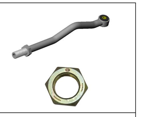
Thread the passenger side track bar section into the threaded connector (1302030-4).
