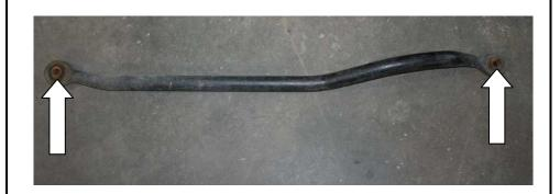
Locate the passenger's side track bar section (#1302030-2). Thread the 90°grease nipple (#1302056) into thread port on the side of the unit.
