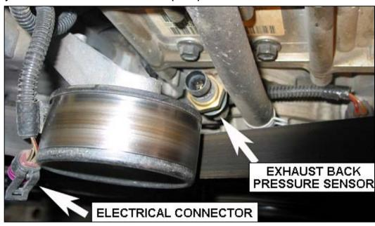
connector. Run the remaining wire away from the belt and the pulley and use the nearest engine bolt as a ground.
