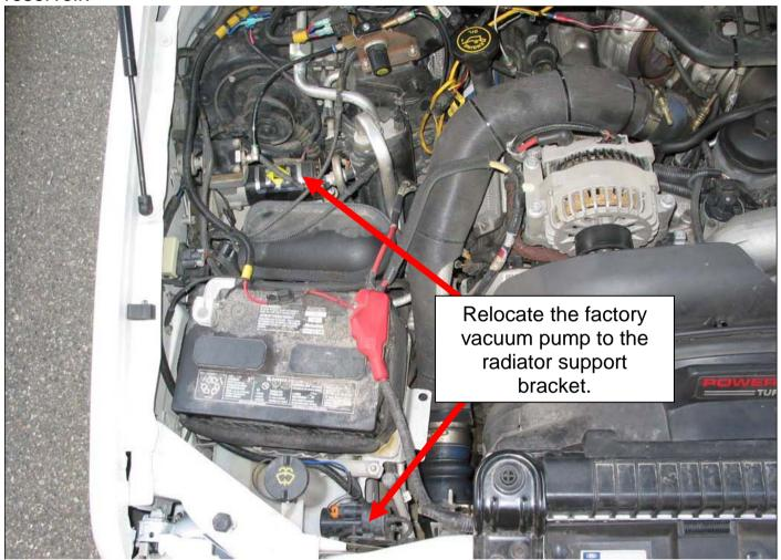
Remove the electric vacuum pump from the stock mounting location and re-install it on the new mount provided. Trim the rubber ends on the three vibration dampers to clear when reinstalling. Install on the right hand side of radiator support bracket with the two bolts and washers provided.
