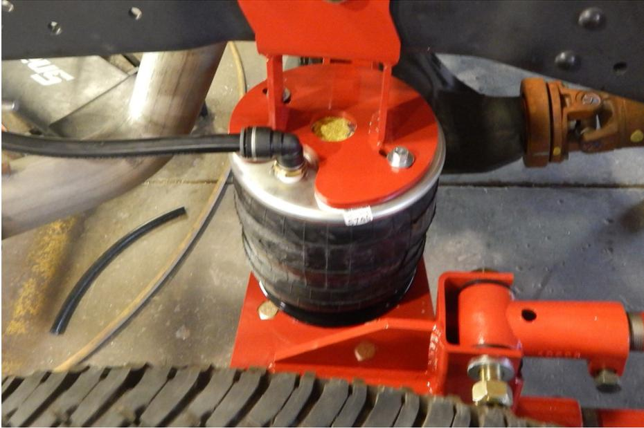
8. Locate the 5748 air bags (part# 5748), 2 accumulator air tanks (part# 21002) and 3/4" air line. The air bags fasten in place with two 3/8x 1" bolts, flat washers and lock washers to the upper bag mount and a 5/8" nut and lock washer on the bottom bag stud. Insert the 90 degree air fitting and tighten into the top of the bag. Use Tef-
