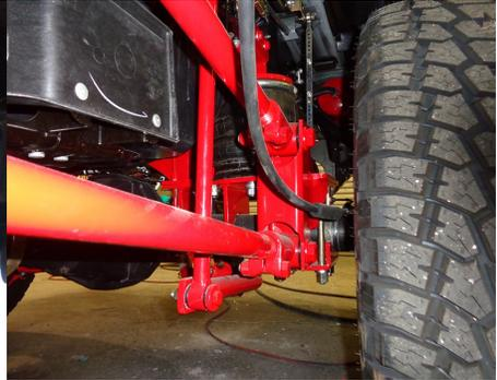
7. Remove the bump stops on the bottom of the frame. Now locate the upper air bag mounts (part# 70507DS and
