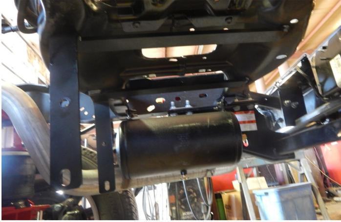
The best place for the Hadley box and air tank is where the spare tire originally went. Use the supplied mounting tabs and weld them to the spare tire carrier. Make sure to use a battery protection device on the batteries or unhook the batteries before welding!
