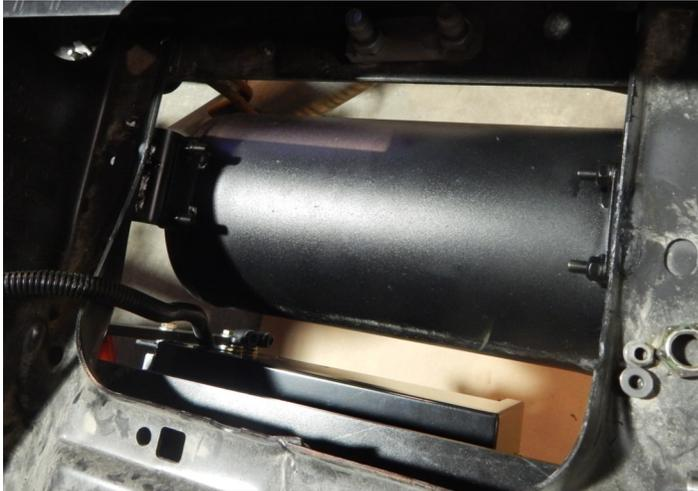
If a spare tire is going to be installed, relocate the drivers side accumulator tank, cut off the leaf spring shackle hanger and make a bracket to mount the box there. Make sure to measure out the box or reinstall the box before fully welding the mounting bracket to ensure its in the correct location.
