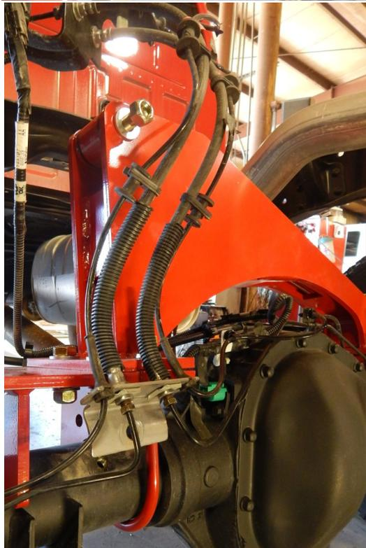
4. Locate the lower pan hard bar (cross member part# 70540). It fastens to the lower bag mounts with two 5/8x2" bolts and one 5/8" u-bolts. Once you get the bolts started you can torque the 5/8" bolts to 150 ft/lbs, including the lower bag mounts and fasten the 5/8" U bolt to 85 ft/lbs.
