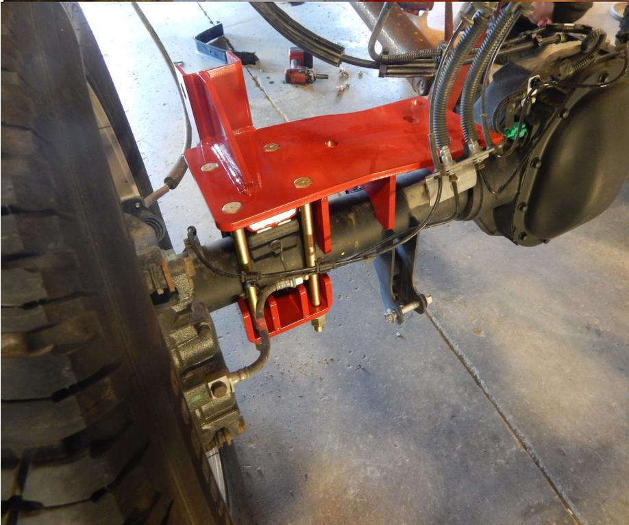
3. Locate the lower bag mounts (part# 70403 DSSRW and 70404PSSRW) and the lower axle clamps (part# 70402 SRW). The axle clamps fit on top of the leaf spring perches and fasten to the axle with the axle clamps and the 5/8x9" bolts. Fasten the bolts finger tight, but do not torque yet.
