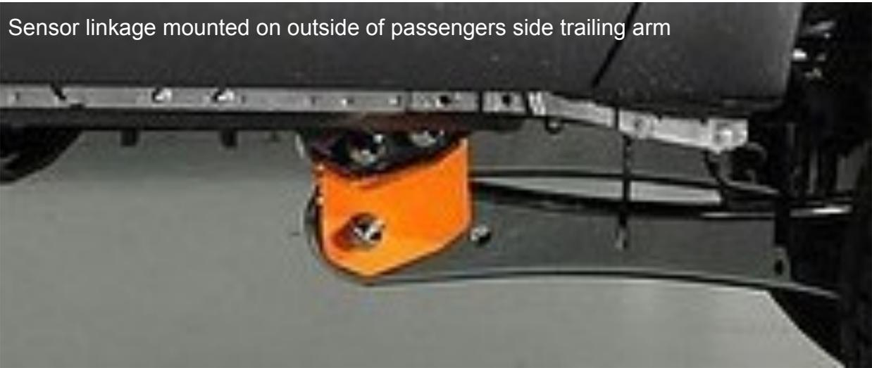
Sensor linkage mounted on outside of passengers side trailing arm
