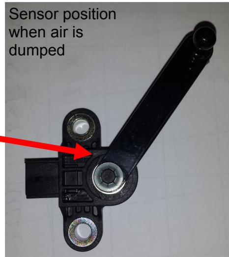
Sensor position when air is dumped
