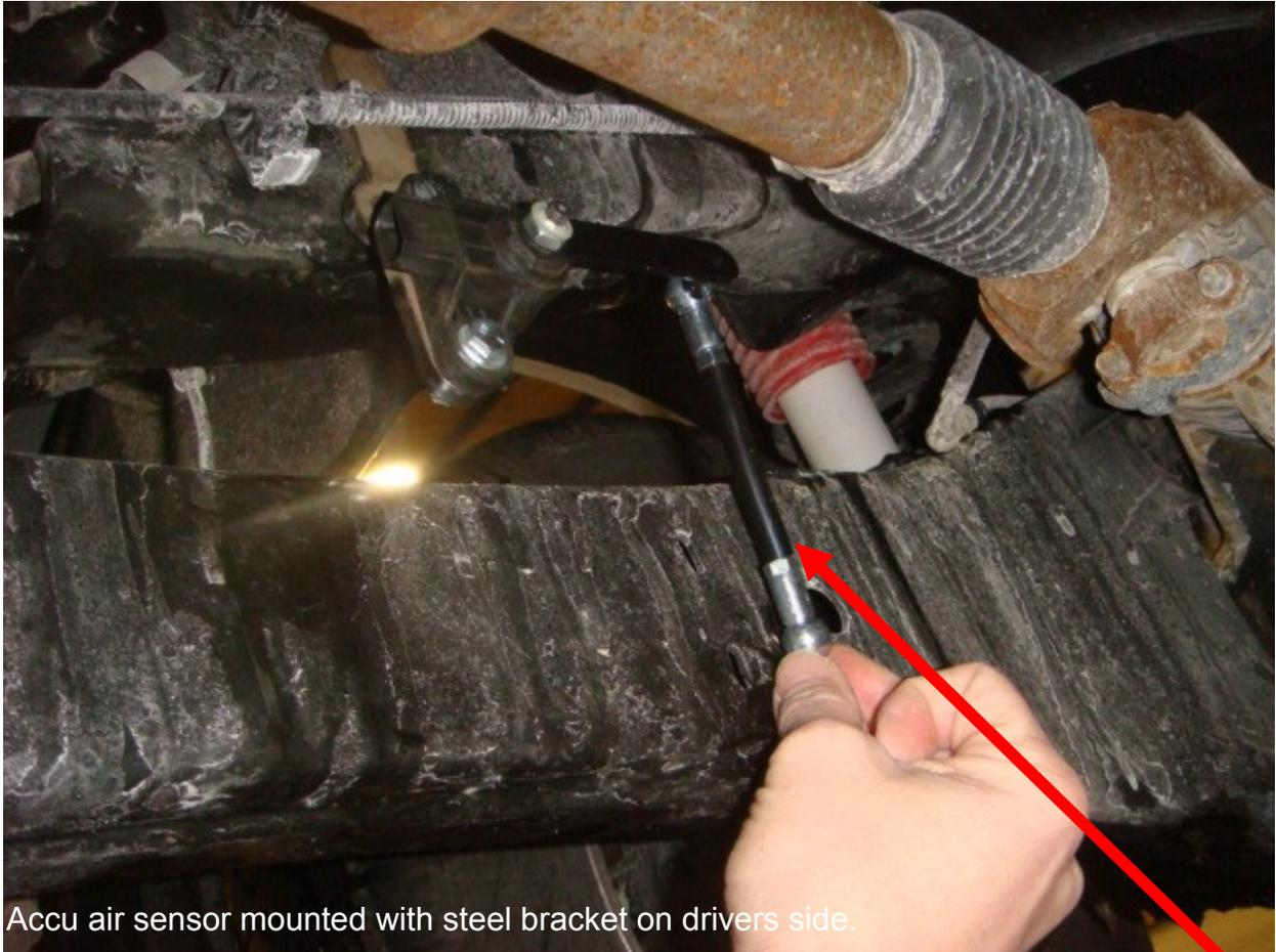
Accu air sensor mounted with steel bracket on drivers side.
