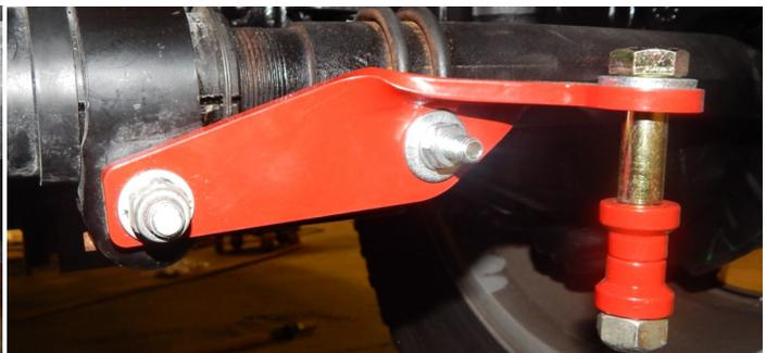
9. Locate the upper shock mounts (part# 17139). They fasten into the original upper shock hole in the spring bucket. Remove the upper rubber mounting brackets from the factory shocks and use them and the M12x70 to fasten into place. Insert the bolt so the threads are up. Torque this bolt to 65 ft/lbs. Now install the shocks with the 1/2x3" bolts. Torque these bolts to 85 ft/lbs. Depending on what brand of shock is used, you may need spacers or washers to center the shock.
