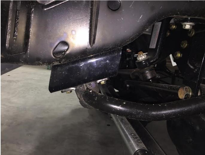
11. Locate the extended brake lines. You can install them now. It is personal preference if you want to remove the steel mounting bracket or use it. Some trimming will be required to the bracket if you want to use it. It will fasten to the lower bag mount with the 1/4" bolts.
