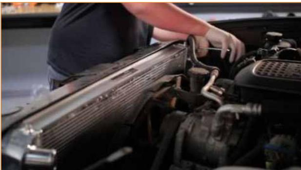
4. Now reinstall the transmission cooler lines. These lines feature a quick disconnect. The clips that were removed earlier need to be reinstalled and the lines can then be pushed back into the radiator. An audible click will indicate that the lines are properly seated, and the radiator and clips. Once this is done slide the dust shields back over the fittings.
