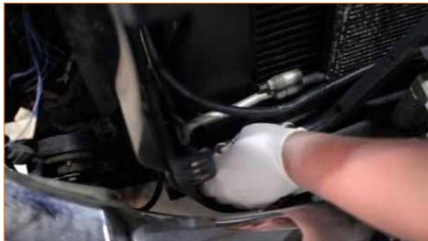
**17.** Install the two 10mm bolts securing the hood release frame to the upper radiator support bracket.
