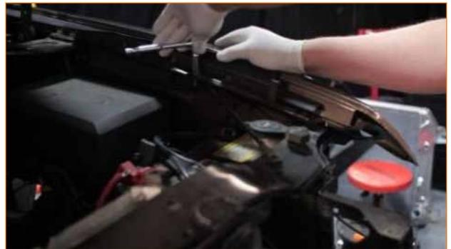
31. Remove the six 10mm bolts that hold the upper radiator support beam to the lower portion of the radiator support.
