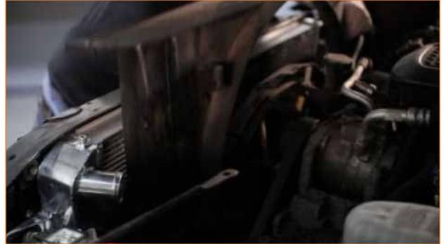
6. Secure the upper fan shroud to the lower fan shroud using four pop clips.
