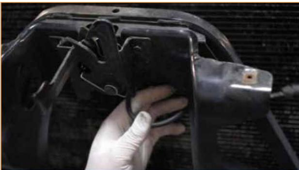
21. Remove the hood release frame assembly from the front of the truck.
