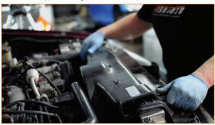
**8.** Install the four 10mm bolts securing the upper cooling fan shroud to the lower shroud
