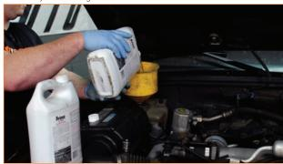
11. Start the vehicle and turn the heat on high. Let the vehicle run for 10-15 minutes while you check for any leaks. You may need to top off the fluid during this time. If you have a vehicle equipped with an automatic transmission, check the fluid levels and refill accordingly.
