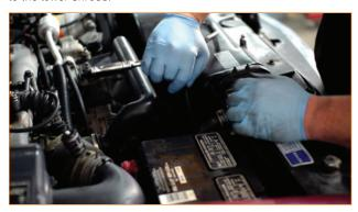
$\bf 9.$  Install the three 10mm bolts holding the upper fan shroud to the radiator support.
