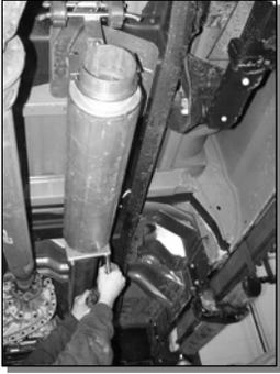
2. Install the **Muffler** over the **Extension Pipe**. The **Hanger Clamp** is used at the connection between the **Muffler** and the **Extension Pipe** and installed into the OEM rubber hanger at this position. Install the “**T**” **Hanger Clamp** into the two OEM rubber hangers located above the outlet of the **Muffler**. **See Figure 3.**
