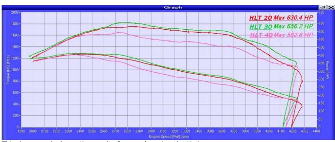
This dyno graph shows the result of over advancing the timing. (All other parameters have remained unchanged during these runs!)
