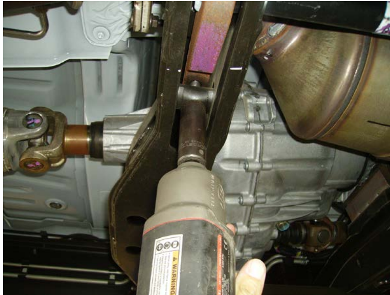
Figure 1: remove torsion bar adjusting bolt
