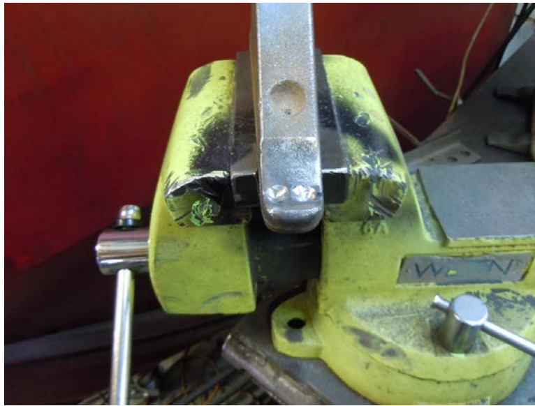
Figure 17: using a drill motor and 1/2" drill bit, drill only 1/8" deep from the tip so create 2 counter sink spots.
