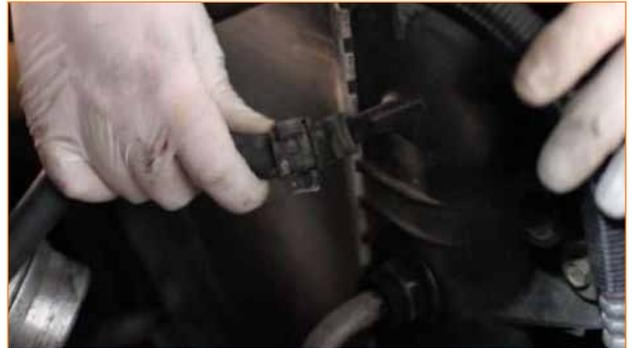
27. Unseat the lower fan shroud from the radiator by pulling upwards on the tabs on each side of the shroud.
