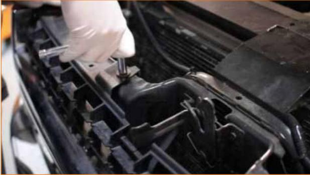
14. Carefully unclip the grille from the front of the truck. The plastic can be quite brittle, even in newer-model trucks.
