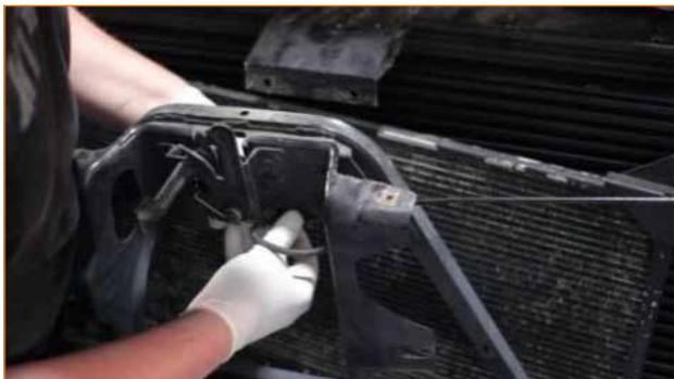
15. Install the two 10mm bolts that secure the upper AC condenser brackets to the radiator support. Do not tighten these bolts at this time.
