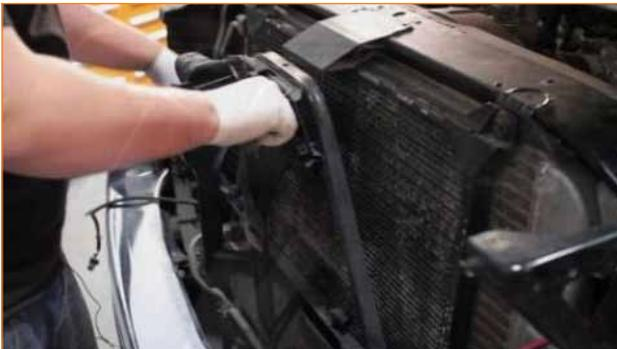
22. Remove the two 10mm bolts securing the AC condenser to the upper radiator support.
