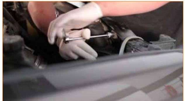
30. Remove the 10mm bolt that secures the fender support bracket to the radiator support. The support bracket bolt located on the fender must be loosened so the bracket can slide away from the radiator support and towards the engine.
