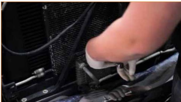
19. Tighten the two 10mm bolts securing the upper AC condenser brackets to the radiator support.
