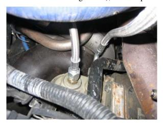
13. FOR 2ND GEN TRUCKS ONLY: The following picture shows how the oil drain on all 2nd Gen 1994-2001 trucks should be routed, then the lower end of the oil drain simply attaches to the block insert (included with the kit) in the front passenger side of the block.
