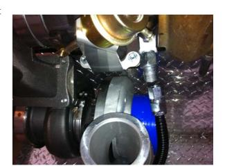
8. Find the 4.4 inch v-band clamp that connects the small turbo to the hot pipe (elbow). Remove the nut off the vband clamp or simply unhook the bolt so the clamp is open, and set the open clamp on the rear of the small turbo's flange where it will mount.
