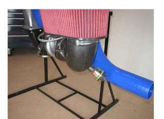
tubes to get the filter in the right place. Make sure the hood does not crush the filter.
