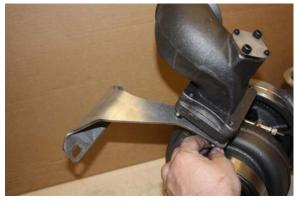
Leave the two bolts going through the bracket just barely loose, so they can be adjusted, once the top is on. All of the bolts going through the support bracket should be a little loose to allow the lower turbo to be adjusted to align the hot pipe with the top turbo. If necessary the bracket can be slightly flexed during the installation if the bolts are a little loose, then tightened when everything is aligned.
