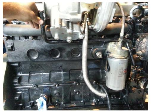
Top Turbo Oil Drain will go in as shown here, on all trucks that have the front oil port in the block (1997-2013 trucks).
