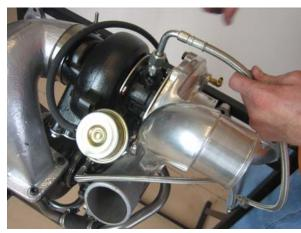
Next, remove one of the oil plugs from the top of the oil filter mount, and screw in the provided fitting (should be at the end of the steel braided oil line from the large turbo), then couple the oil line to that fitting.
