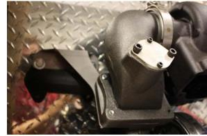
Tighten the bolts most of the way, but do not completely tighten theses two bolts...yet.
