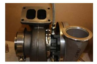
5. Place this large turbo, elbow and support bracket assembly in the truck. Simply and carefully set this whole assembly on the truck frame. Do not attach the exhaust yet. **Be very careful not to damage the steel braided oil supply line or the oil drains.** (Picture below shows HT3B turbo, for S400 turbo air outlet will go up.)
